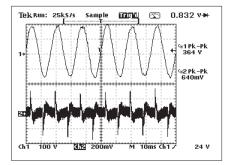
To safely acquire floating measurements with TekScope, use the P5102 high voltage probe (10X attenuation)
